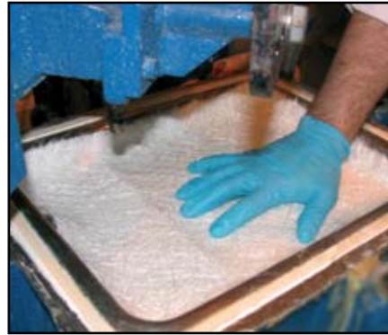
Reinforcement being laid in the press
