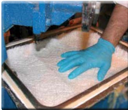
Reinforcement being laid in the press
